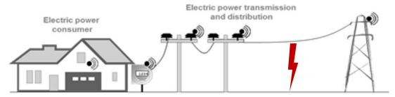
Implementation of a monitoring system through distributed devices paving way to a **fully digitalization of the LV grid** and the implementation of automation procedures based on "information exchange among fault detectors"
