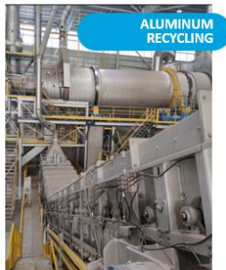
TRANSPORT & DIRECT CHARGING OF HOT SHREDDED SCRAP FROM THE DECOATER TO THE MELTING FURNACE
