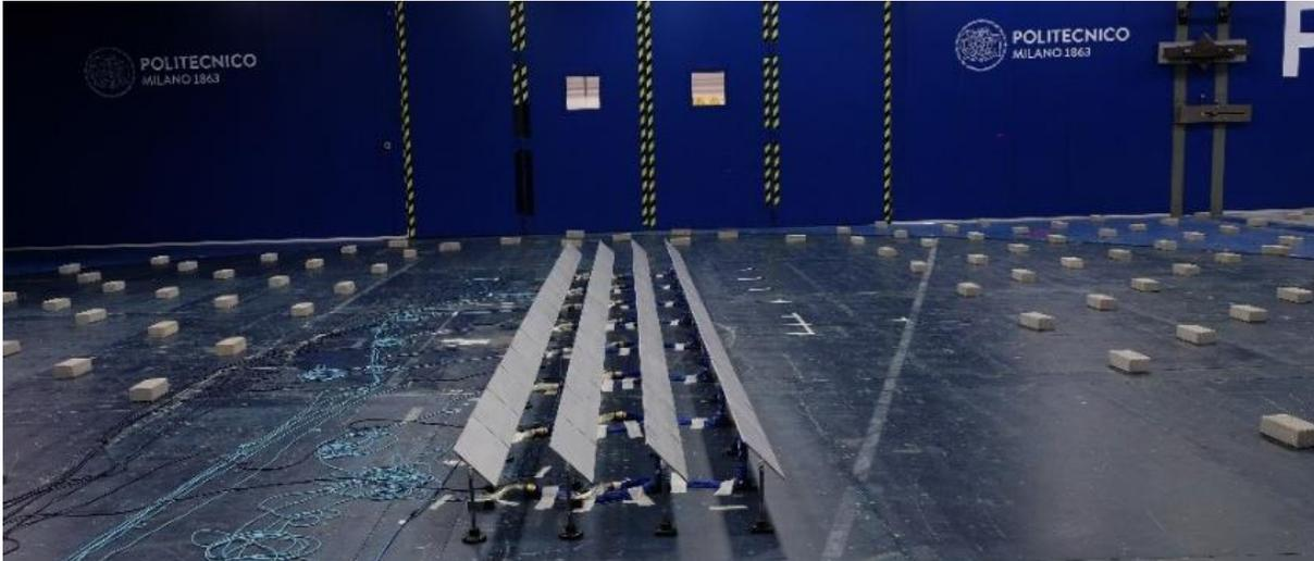
A photograph showing a PV tracker system in a wind tunnel. The tracker is a long, narrow, rectangular structure made of a light-colored material, possibly aluminum or steel, mounted on a blue base. The background is dark, and the floor is light-colored. There is a blue smoke visualization around the tracker, indicating the flow of air around the structure. The background wall has the logo of Politecnico di Milano.
