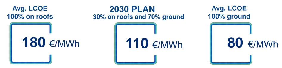
Rooftop PV plants show a power generation cost that is more than double of the cost related to ground-mounted plants. The 2030 Plan scenario shows savings of over € 20 bn on the electricity generation's side (2024-2030) compared to a 100% rooftop-mounted scenario.
